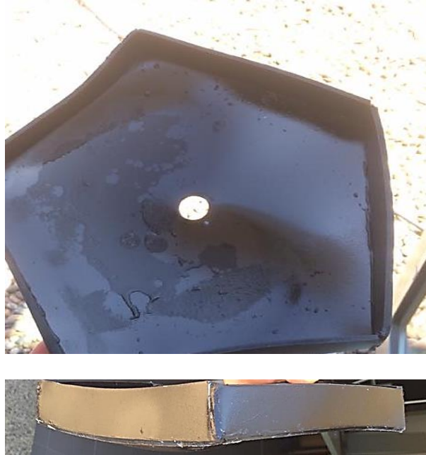
Fig. 54: (A) Top view of the deformed black container and (B) Side view of the deformed black container
