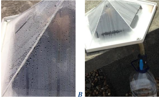
Fig. 8 Condensation Process (A) Collecting the water (B).
