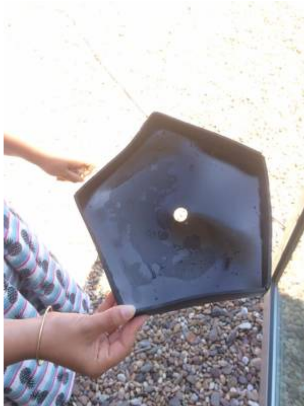
Figure 55: Deformation of the container
