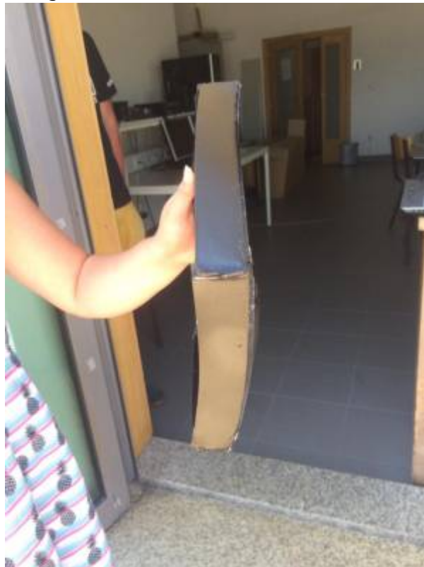
Figure 56: Deformation of the container
